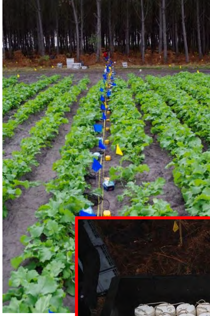
(b) Line array with GFZ geophones (c) Vibrometer source (> 15 Hz)
