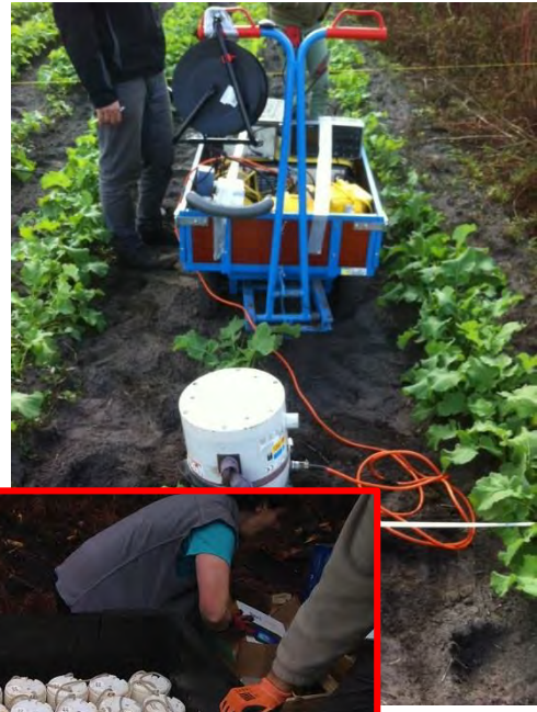
(b) Line array with GFZ geophones (c) Vibrometer source (> 15 Hz)
