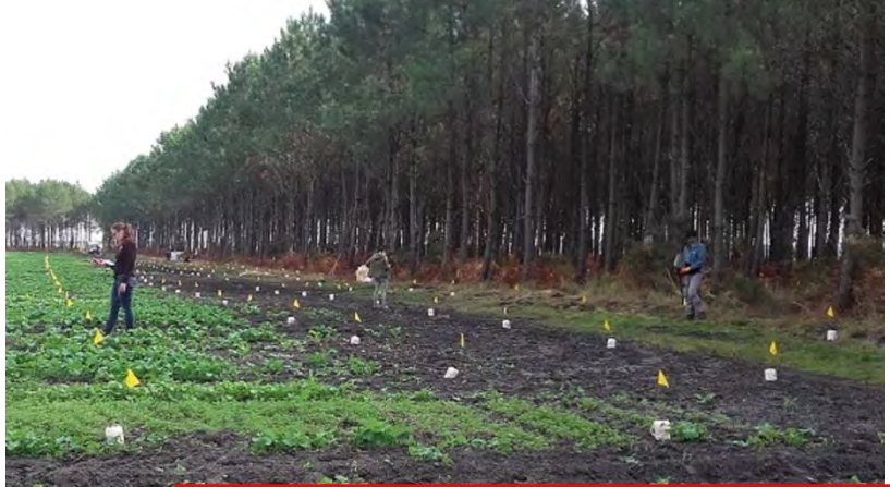
(a) 2D Seismic array with Z-land geophones
